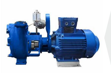
Suction port Threaded - 3" ISO 228 (BSP) Delivery port Threaded - 3" ISO 228 (BSP) Qmax 80 m<sup>3</sup>/h - 1333 l/min (352 USgpm) Hmax 21 m (69 ft) Solids handling 28 mm (1,1") Motor power 4 kW - 5,5 HP Motor type **IEC** standard **Cast iron frame** Motor brand CEMP Weight 122 kg (269 lb)
